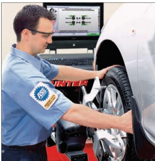
*Using DSP500XF Cordless Sensors, technicians make only one trip around the car to compensate each sensor as it is mounted.*
